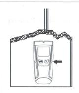
Continue scanning beyond the marked spot to detect width of target. If target is wide, reverse to locate and mark the other edge. Avoid sawing or drilling between the two marks. Widths will vary from single peak for narrow rebar to wide area for metal studs, I beams, junction boxes,
